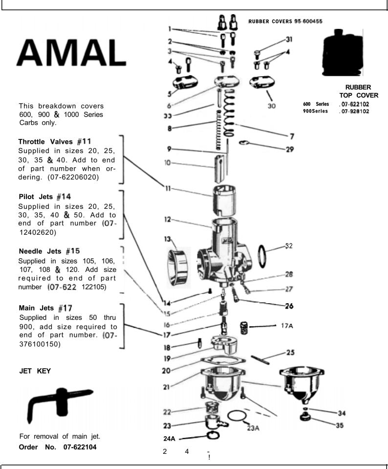
Note: 07-622/122 Needle Jet, 07-622/128 Jet Holder & 07-622/124 Needle must be used as a unit.
